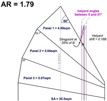
The Sheet 1 of the AR=1.79 sailplan. All sailplans use the same max/min halyard angles and drift
