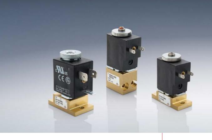
Series AP directly operated 2/2-way proportional solenoid valves, NC, with nominal diameters range from 0.8 to 2.4 mm, can be used where an open loop flow control is required, with gas mixtures, to control free flows or blows, or emptying chambers using vacuum.
