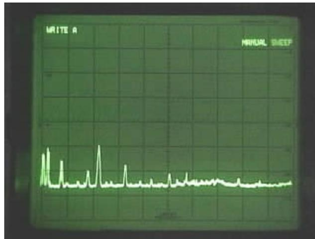
The center frequency for the two pictures above is 1.7 MHz. Insertion loss in the 160 Meter band is less than .8 dB at the very low end of the band (1.8 MHz) and less than .5 dB at the high end (2.0 MHz) of the band.
