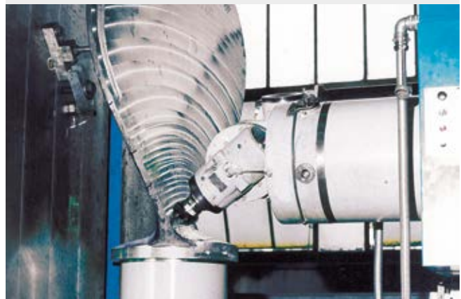
Horizontal milling-boring machine for propellers
