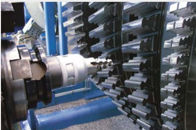
Rotor slotter for turbine rotors
