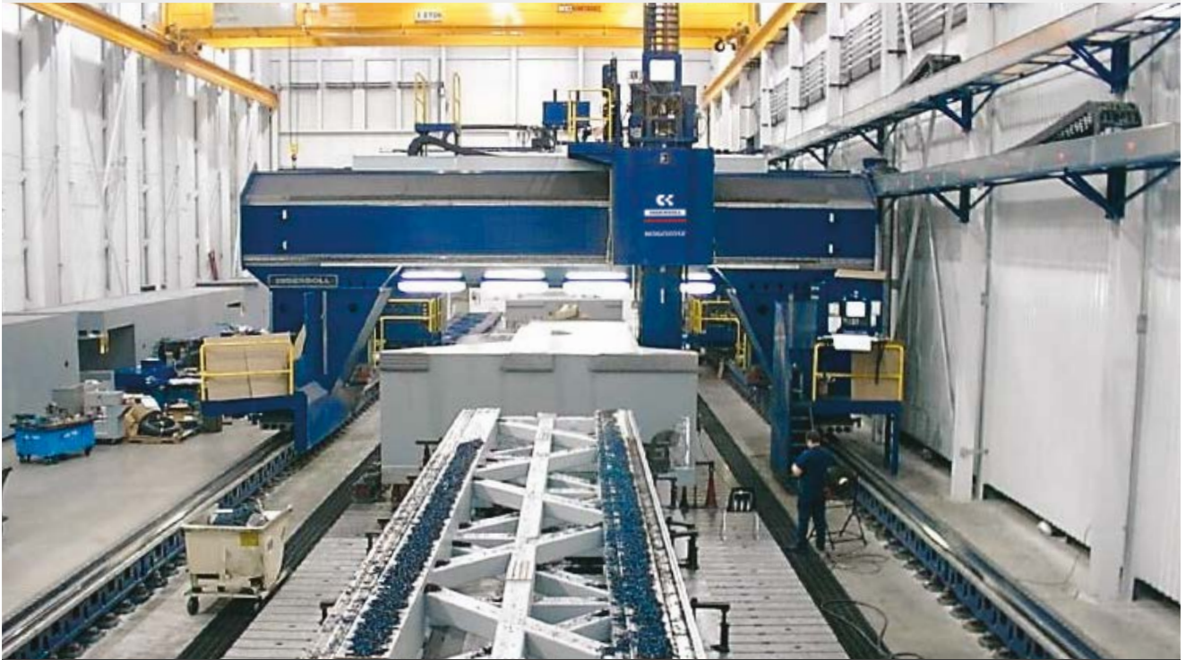
Horizontal milling-boring machines for general mechanic components
