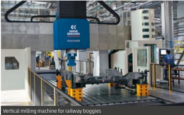
Vertical milling machine for railway engines
