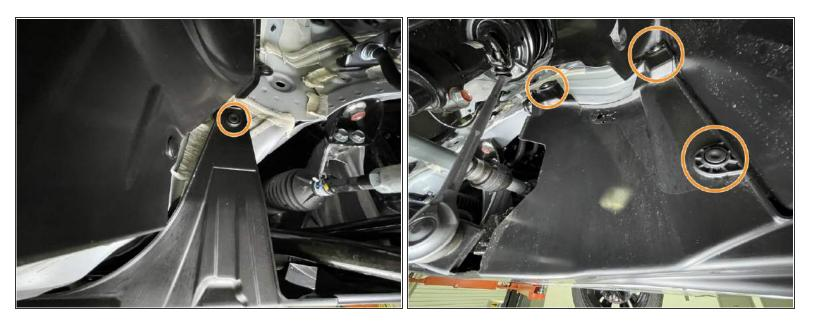
Use a large flat head screw driver or prying tool to remove the four (4) push-clips from each front wheel well
