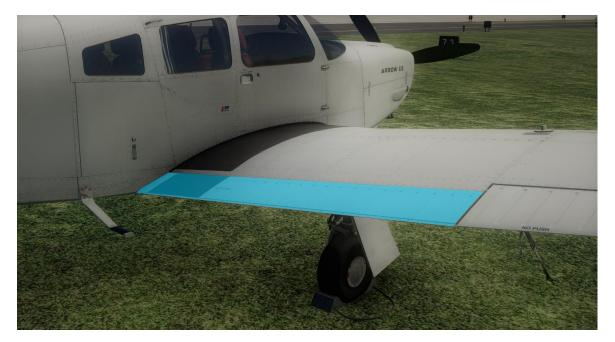
Flaps are important parts of a wing that can be deployed when the aircraft is taking off or landing, or travelling at a very slow speed. In simple terms, they change the aerofoil shape of the wing overall, by moving and lowering an entire section of wing. This makes the wing generate more lift at a slow speed, allowing the
