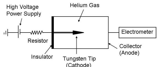
**Fig. 1.** Apparatus for measuring helium ionization. To protect the tungsten tip from ohmic heating, a 100-G $\Omega$  resistor was connected to the field emission tip. A collector made of copper was used to measure the current with an electrometer. The tungsten tip and the collector corresponded to the negative electrode and the positive electrode, respectively. The distance between the field emission tip and the collector was 1 cm.
