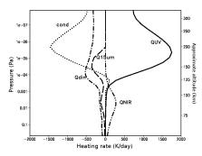
Figure 3: Balance between different heating/cooling terms for perihelium conditions.
