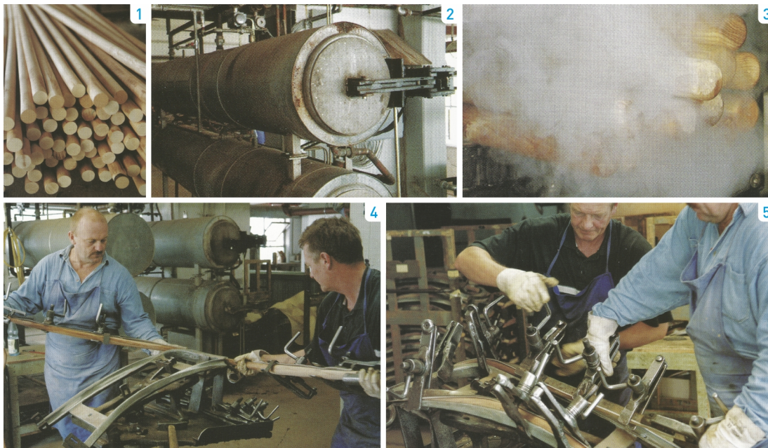
Figure 39. Steps in the bending of a back-rear leg unit (adapted from Thompson, 2007, p. 200)
