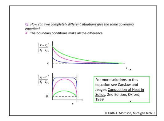
Unsteady State Heat Conduction in a Finite Slab
