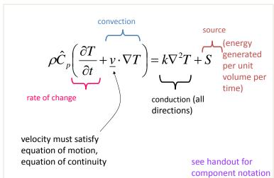
Equation of energy for Newtonian fluids of constant density,  $\rho$ , and thermal conductivity, k, with source term (source could be viscous dissipation, electrical energy, chemical energy, etc., with units of energy/(volume time)).
