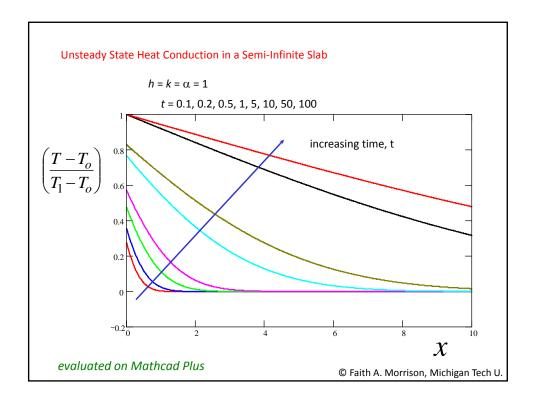
How could we use this solution? Example: Will my pipes freeze?
