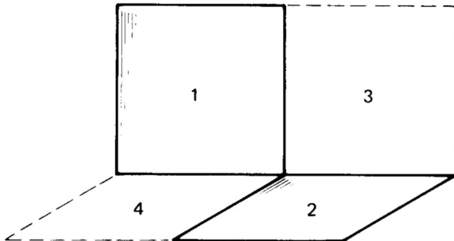
**Figure 10.12** Radiation between 2 offset perpendicular squares.
