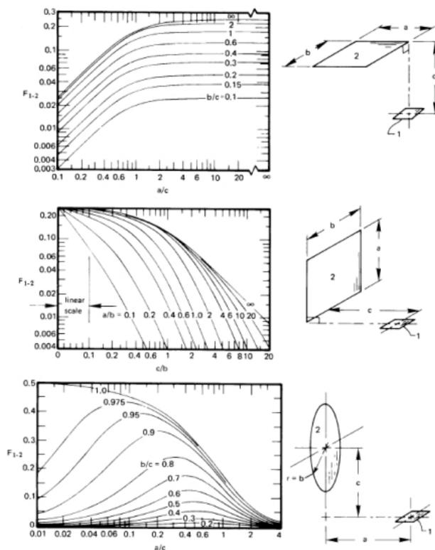
**Figure 10.10** View factor for 3 very small surfaces "looking at" 3 large surfaces.
