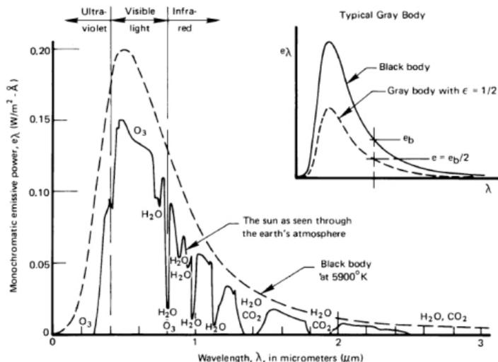
**Figure 10.2** Comparison of the sun's energy as typically seen through the earth's atmosphere with that of a black body having the same mean temperature, size, and distance from the earth.
