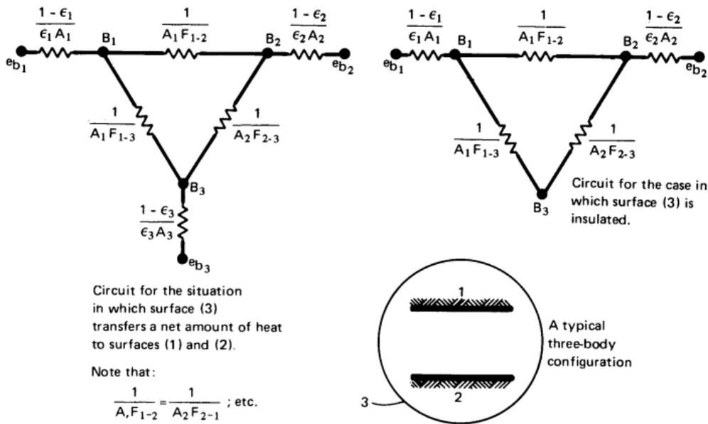
**Figure 10.15** Electrical circuit analogy for radiation among 3 gray surfaces.
