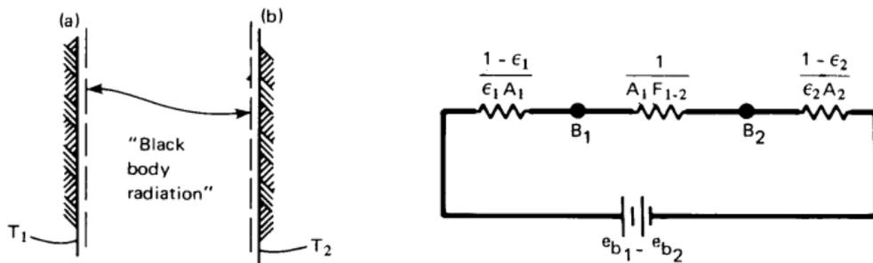
**Fig. 10.13** Electrical circuit analogy for radiation between two gray infinite plates.
