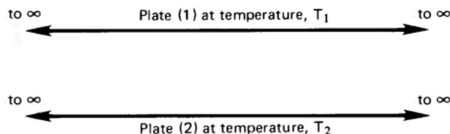
**Figure 10.5** Heat transfer between two infinite parallel plates.
