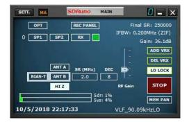
Figure II.7 ~ SDRuno Main window shows general and common receiver settings including antenna port, RF gain, sampling rate and decimation. Also, the receiver is started and stopped and virtual receivers are assigned from this window. Only one virtual receiver was used during this propagation study. The two horizontal meters at bottomleft indicate the PC system and software loads. In this case, the SDRuno software added 1% to the overall system load of 4%.
