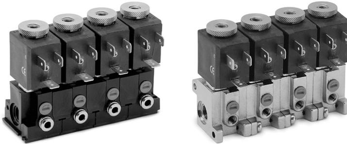
Series A solenoid valves are of the directly operated type and can be used with dry or lubricated air. They are available in the 2/2 and 3/2-way versions with normally closed (NC) or normally open (NO) operation. As shown in the following tables, they are supplied in different versions according to the type of body, threaded ports and orifice. They can thus satisfy various operating and installation requirements.
