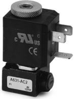
Ideal for direct installation on manifold by means of 2 screws. Seal ensured by 2 concentric O-Rings that allow 360° body orientation. Equipped with a bistable manual override.
