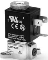
Equipped with a bistable manual override. Ideal for direct installation on manifold by means of 2 screws. Seal ensured by 2 concentric O-Rings that allow 360° body orientation.
