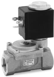
These solenoid valves have a solenoid protection system suitable to be used in particularly humid environments and in harsh conditions. The system consists of two gaskets placed above and below the coil and a lock nut that integrates the upper gasket. The standard diaphragm valve supplied is in NBR. On demand it can be supplied in FKM or EPDM.
