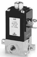
These solenoid valves are equipped with a manual override and are available with G1/8 inlet ports and with G1/8 outlets or with a diameter 4 cartridge. The body is supplied complete with screws and O-ring.
