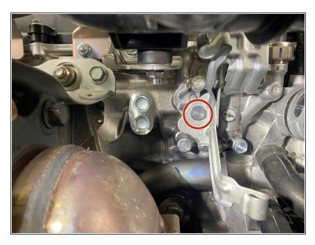
Bolt the secondary O2 sensor wire harness support bracket back in place. Torque bolt to 80 in-lbs.
