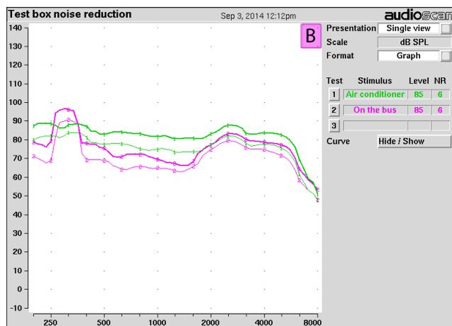
When the noise management strategy is enabled, an average of 6 dB noise reduction is noted when ‘Air conditioner’ and ‘On the bus’ signals are delivered to the hearing aid. Other noise reduction stimuli available in this system include ‘Vacuum’ and ‘Multi-talker Babble’.
