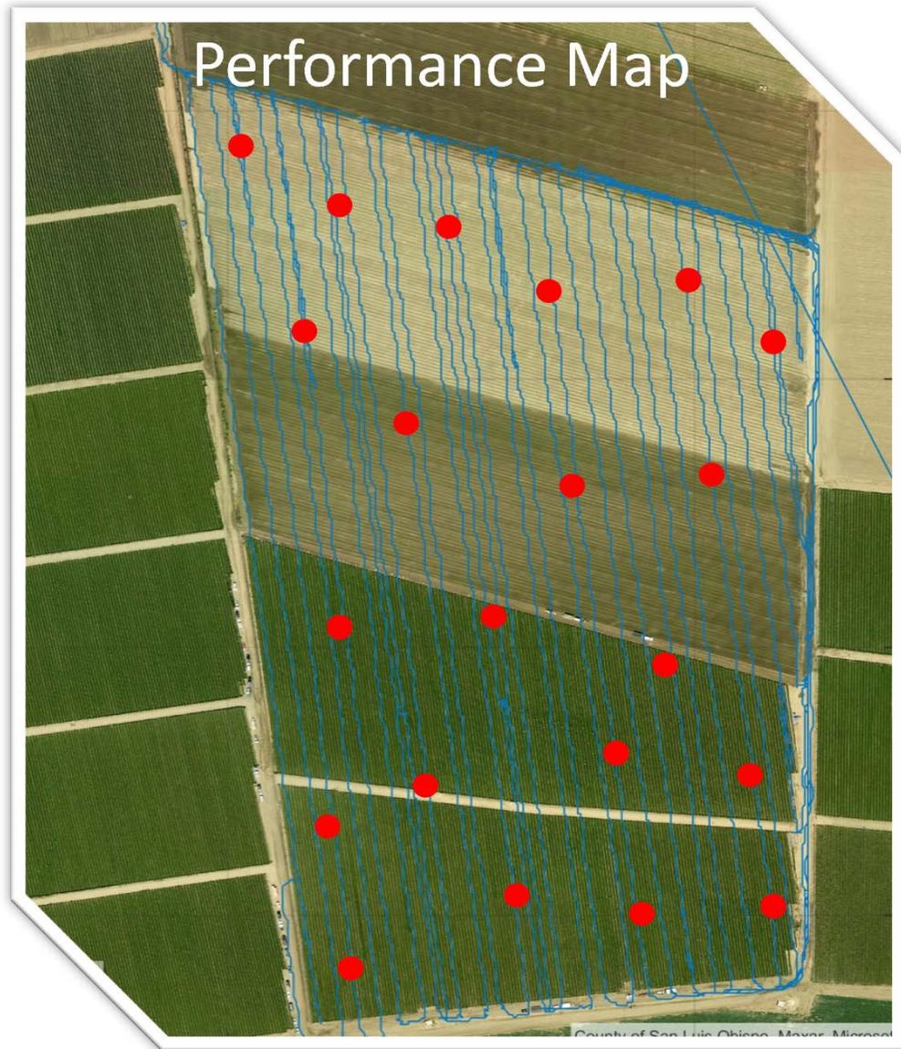
**Figure 1.** The amount of Lygus removed, tractor speed, vacuum air flow, and vacuum height above canopy are measured. The tractor path is shown as blue lines and measured parameters that exceed recommended thresholds are shown as red dots.
