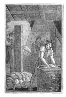
The **dyer** used mainly vegetable dyes to add colour to either wool or woven cloth. After the wool had been cleaned, the dye was applied by soaking the wool or cloth in a brass or copper cauldron.
