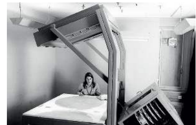
Figure 4: A “scanner” analyzes a bubble chamber photograph.
