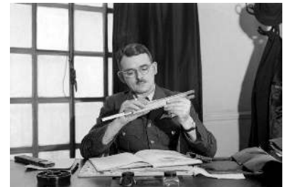
Before computers and calculators became widely available, the slide rule was widely used for calculations involving logarithms or trigonometric functions.
