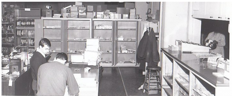
Figure 5.16: In the days before files were stored on disks, students delivered stacks of punched cards to counters like this one in the the basement of the UNC Physics building. Computer operators loaded the stacks into readers, and the program's output was printed (sometimes hours later) and dropped by the operator into a bin, until the student came by to pick it up.
