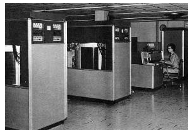
Figure 13.47: The two closet-sized boxes in the foreground are IBM 350 disk drives, introduced in 1956. Each drive can hold a whopping 3.75 Megabytes of data. That's about the size of a single photograph from a modern digital camera.
