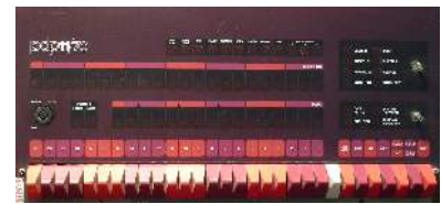
Figure 13.1: The front panel of a DEC PDP-11/70, showing the switches that were used to load a binary starting address into the computer’s memory.
