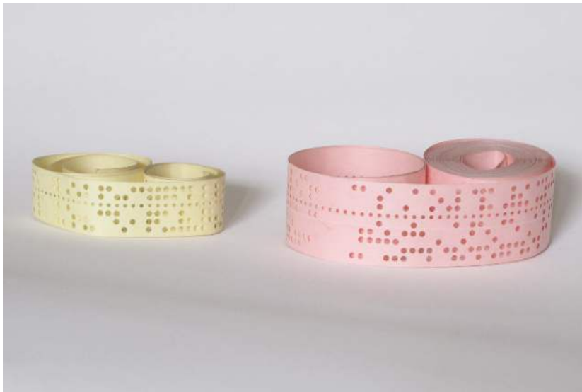
Figure 13.39: In the past, data was sometimes saved on paper tapes like this. Each line (vertical column in this picture) represents a binary number. A large punched-out hole represents a 1 and the un-punched spaces are zeros. (Ignore the line of small holes. That's for moving the tape.) The right-hand tape in this picture is written using 7-bit ASCII characters. The bottom-most position in each line is a special "parity bit" which isn't part of the character but is used for error-checking. The other bits can be read from bottom to top as a binary number representing an ASCII character (see the table in Figure 13.9). The visible part of the right-hand tape says: 10.1 TYPE"DO YOU LOVE ME?" Let's hope the poor programmer wasn't disappointed.
