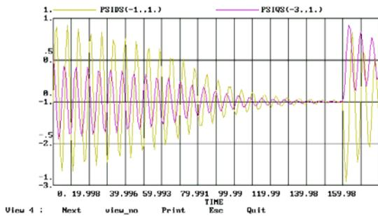
Figure 6: Stator magnetic fluxes
