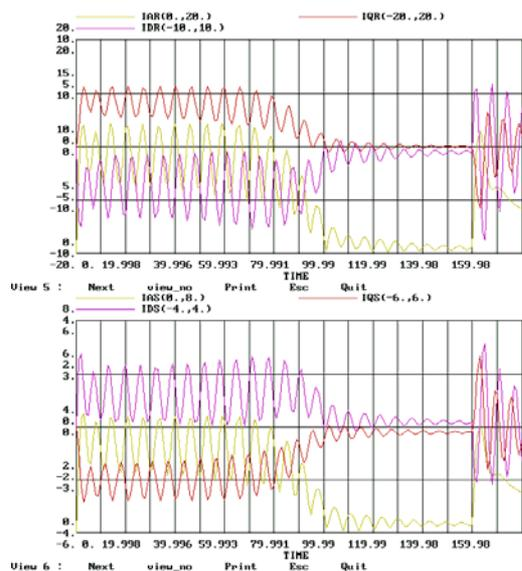
Figure 7: Stator and rotor currents
