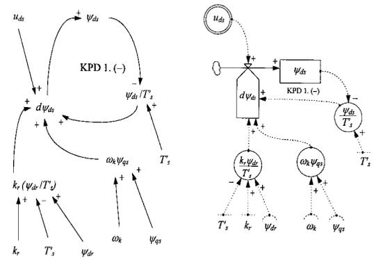
Figure 3: Structural diagram and continuity diagram of the first differential equation of the asynchronous motor condition
