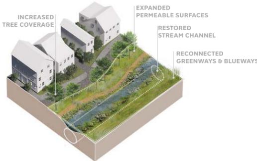
Stream daylighting is the exposure of some or all of the flow of waterways covered in piped or culverts. Stream daylighting and restoration of natural drainage systems can help eliminate flooding issues by re-connecting piped stream channels with the floodplain and re-creating a functioning floodplain and riparian area.
