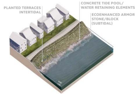
Revetments are hard sloping structures, typically constructed using natural stone, or concrete blocks designed to reduce shoreline erosion by absorbing wave energy and minimizing wave run-up.
