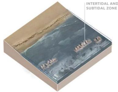
Constructed reefs are subtidal and sometimes intertidal submerged structures that promote marine life and break waves, limiting the wave energy reaching the shoreline. Breakwaters are partially or fully emergent structures that extend above mean high water. They are built with armor units to help attenuate storm waves to improve safety and prevent damage to buildings and infrastructure.
