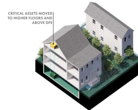
Relocating critical systems to higher floors within structures reduces the impacts of flooding on critical services and reduces recovery times. This tool increases the resilience of essential services to homes and businesses.
