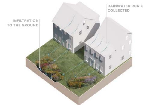
A rain garden collects rainwater runoff from impervious surfaces like roofs, streets, and paved surfaces, thereby reducing risk associated with rainfall flooding.
