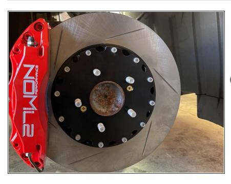
This completes the installation of the physical BBK. It's now necessary to bleed the brakes and bed the brake
