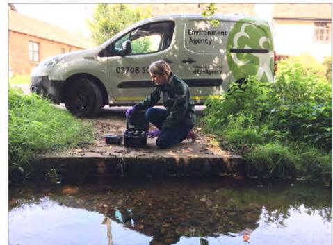
**Left:** Alert Lab being used in a water quality analysis laboratory. **Middle:** The equipment during a field operation, analyzing six samples simultaneously. **Right:** Alert Lab as used by regulatory agency agent in the field.
