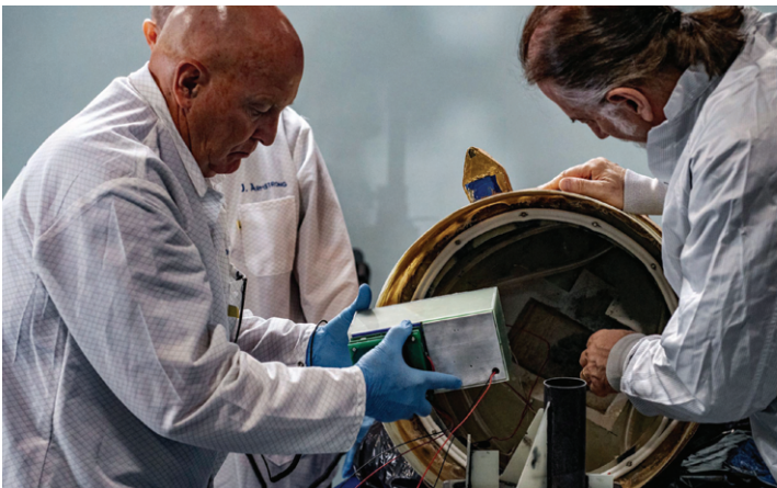
TriSept employees integrate student-built payloads with RocketStar's Cowbell suborbital launch vehicle.
