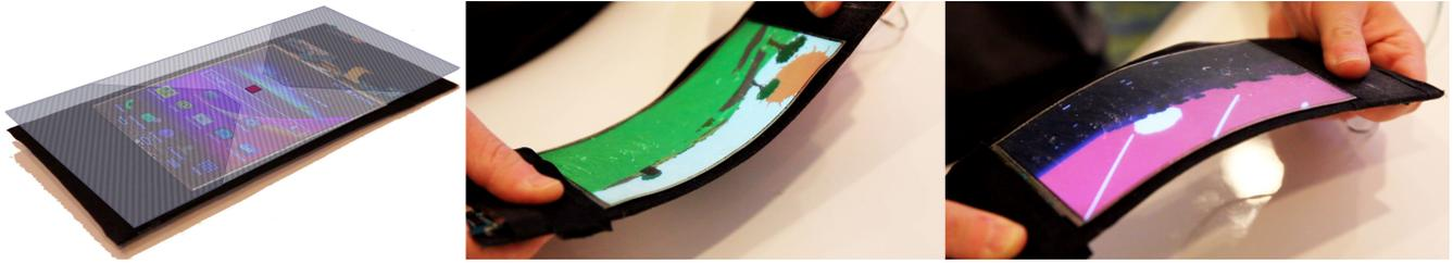
**Figure 2. Left: Prototype with internal structure: Dark gray areas are semi-rigid, light gray areas are flexible. Position and size of strain sensor is indicated by the red square. Middle, Right: ReFlex bending in both directions.**
