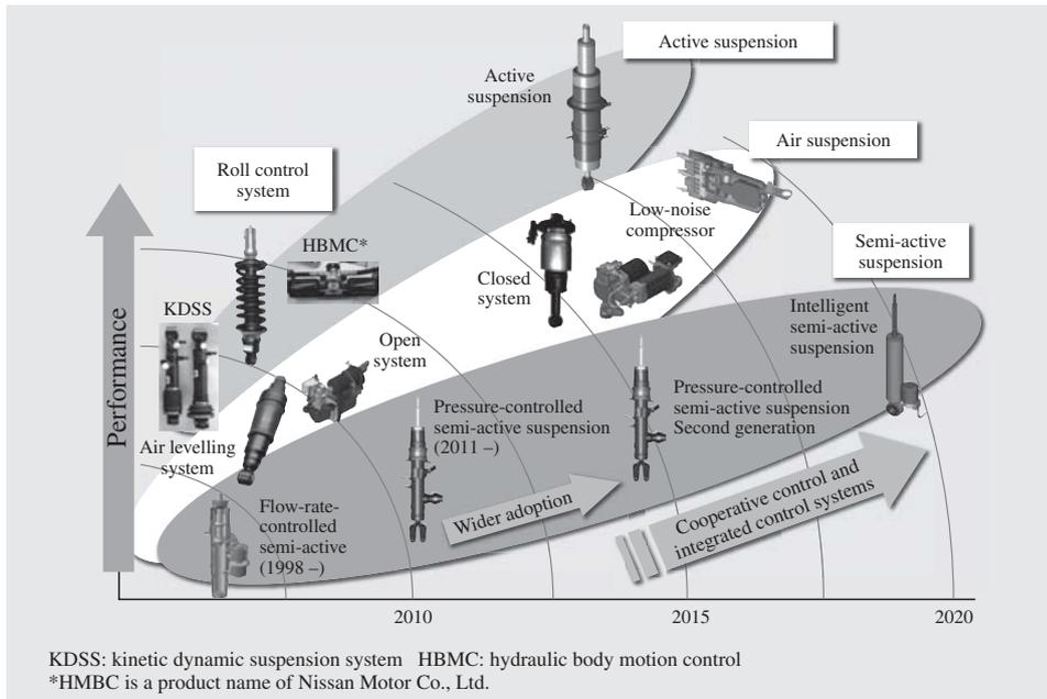
Fig. 5—Roadmap for Controlled Suspension. Use of semi-active suspension, in particular, is extending beyond top-end models to also include small, low-cost vehicles, with performance improvements being achieved through integrated control in cooperation with other chassis control systems.
