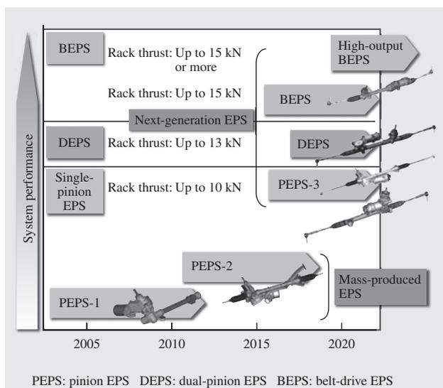
Fig. 8—Roadmap for EPS. In addition to PEPS, Hitachi is also developing DEPS and BEPS to suit a wider range of vehicles.
