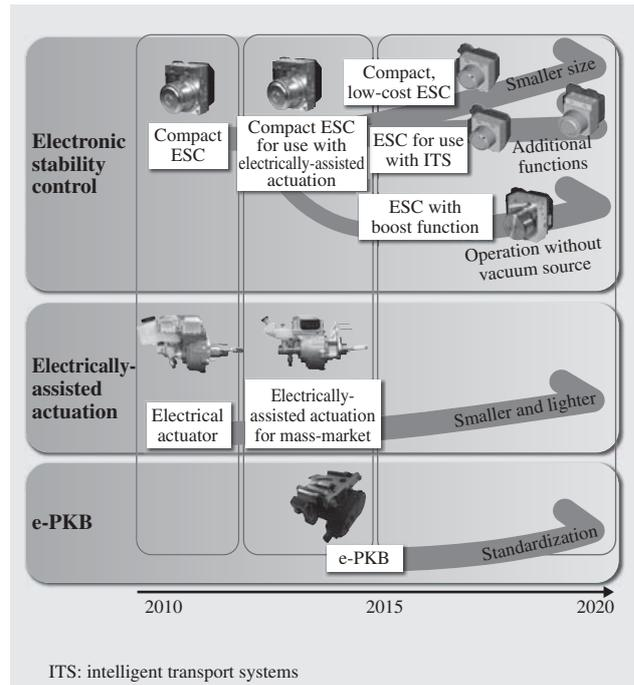
Fig. 3—Roadmap for Controlled Brakes. With a product range that includes skidding prevention systems, electric actuator, and e-PKBs, Hitachi supplies brake systems that cover everything from normal driving conditions to extreme cases.
