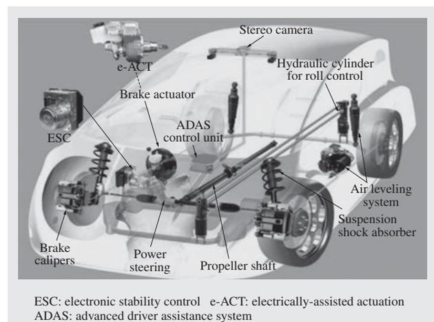
*Fig. 1—Chassis Control System Products. Hitachi supplies a variety of products for chassis systems, which play an important role in determining the driving, cornering, and stopping performance of a vehicle.*
