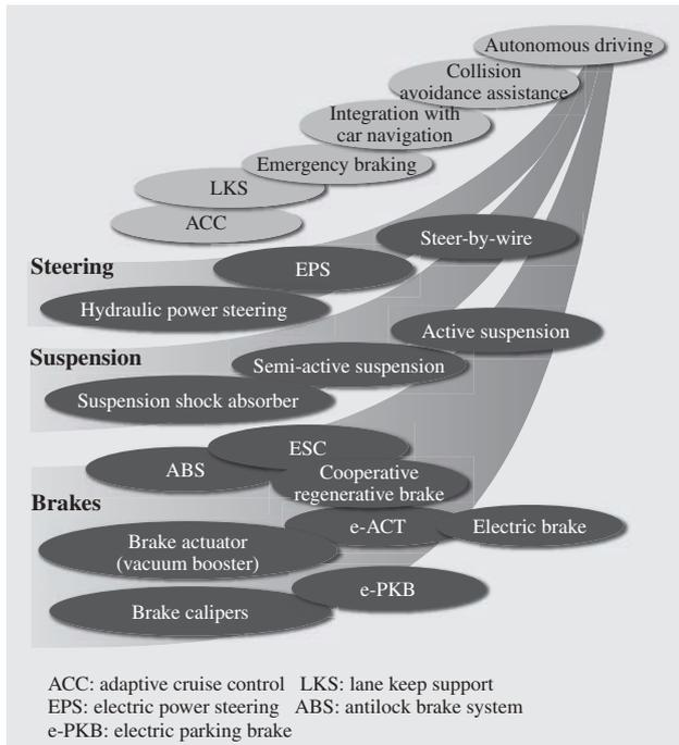
Fig. 2—Advances in Chassis Control Systems. By drawing on technologies it has developed with conventional products to incorporate electronics and electric drive and enhance cooperative control techniques, Hitachi is creating vehicles that are safer, have better environmental performance, and are more comfortable.
