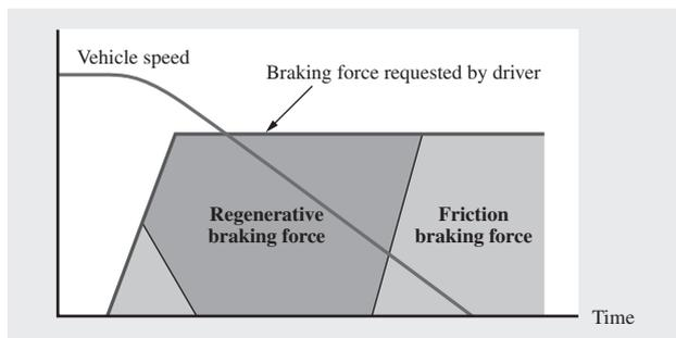
Fig. 4—Cooperative Control of e-ACT and Regenerative Brake. e-ACT works in conjunction with the regenerative brake, adjusting the friction brake and controlling the two mechanisms in tandem to provide the driver with the intended braking force.
