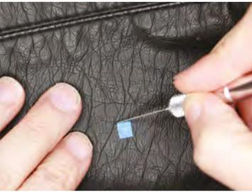
Use a craft knife to cut a square hole at each mark for the NeoPixel to show through, making sure not to cut into the jacket lining. A small square of blue tape works well as a cutting guide.
