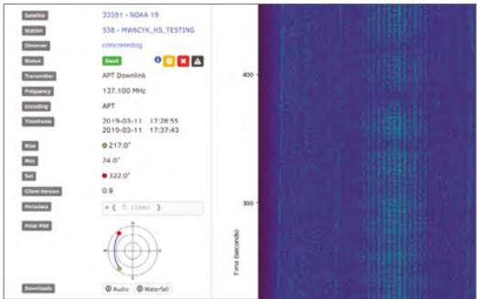
**Figure 3** ♦ Here, we can see a successful observation using the simple SatNOGS test station we built earlier connected to the Slim Jim antenna
