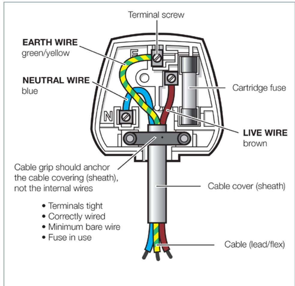
44 For moulded plugs the fuse can be checked. The formal visual inspection should **not** include taking the equipment apart. This should be confined, where necessary, to the combined inspection and testing.
