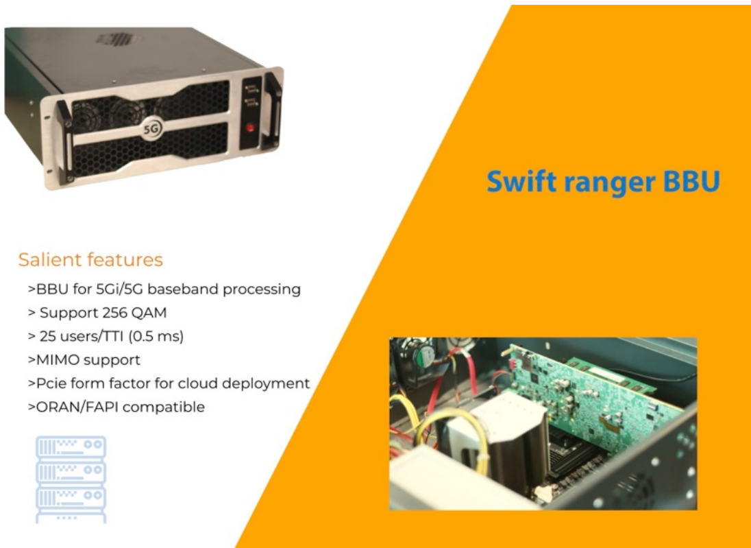
Fig. 2: Baseband unit designed at IIT Kanpur by the group of Dr. Rohit Budhiraja. Also shown is the close-up of the hardware.
