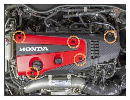
Remove the five (5) 10 mm bolts circled in orange with a 10 mm deep socket and ratchet and then remove the engine cover
