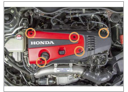
Align the engine cover on the engine, and install the five 10mm bolt with a 10mm deep socket and ratchet
