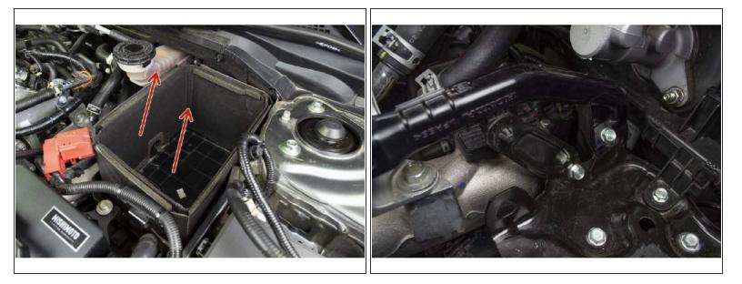
• Remove the battery foam and tray case to reveal the battery bracket.
