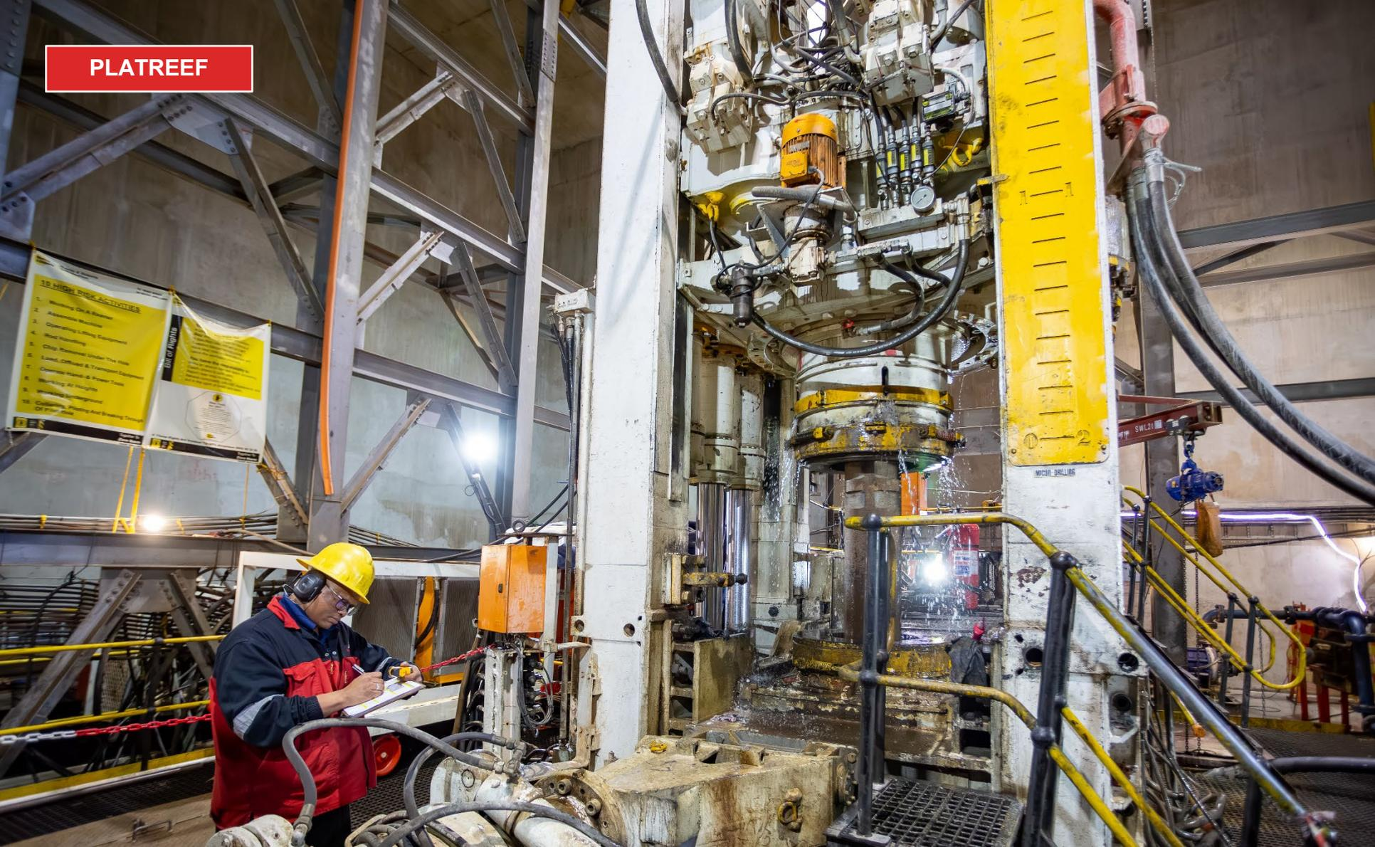
Koos Titus, Shift Superintendent, logging the temperature reading of the raise bore drill at Shaft 2.
