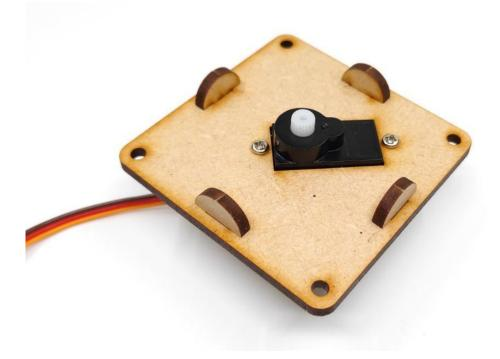
Fix it with M3\*8 screws; as shown in the figure:
