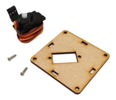
When fixing the steering gear; pay attention to the direction of the steering gear, and the main shaft is in the center of the base.
