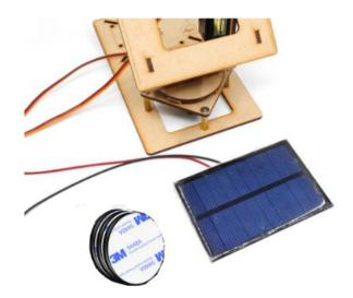
Paste the round double-sided tape on the back of the solar panel
