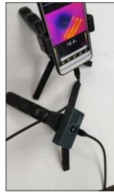
Imager fixed on tripod and connected to Smartphone through extended cable
