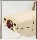
5.安装机轮及起落架 Wheels and landing gear installation
