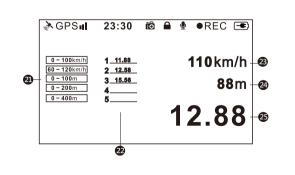
Recording Status (Flashing Red Dot Indicates Recording)
