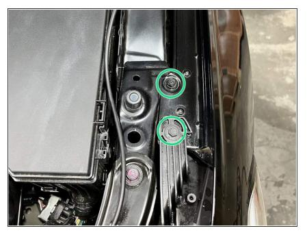
• Use 3/8" ratchet and 10mm socket to remove the two (2) 10mm bolts
