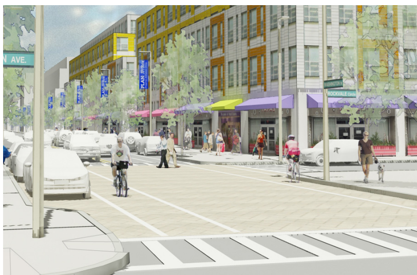
Figure 90. Conceptual drawing looking north on Washington Street near Forest Hills showing enhanced public realm interventions: bike lane, wide sidewalks, curb bump-out, marked crosswalk, abundant street trees. For orientation purposes, note right: Washington Street and Rockvale Circle intersection. Illustrative diagram.
