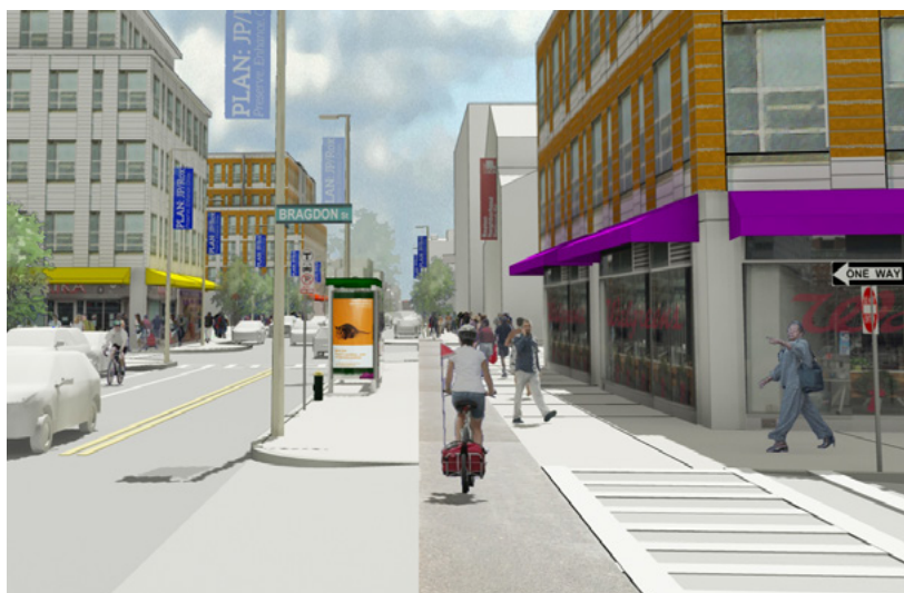
Figure 89. Conceptual drawing looking south on Washington Street near Egleston Square showing enhanced public realm interventions: dedicated cycletrack, wide sidewalks, marked crosswalk, ground-floor transparency. For orientation purposes, note right: Walgreens and BNN banner. Illustrative diagram.
