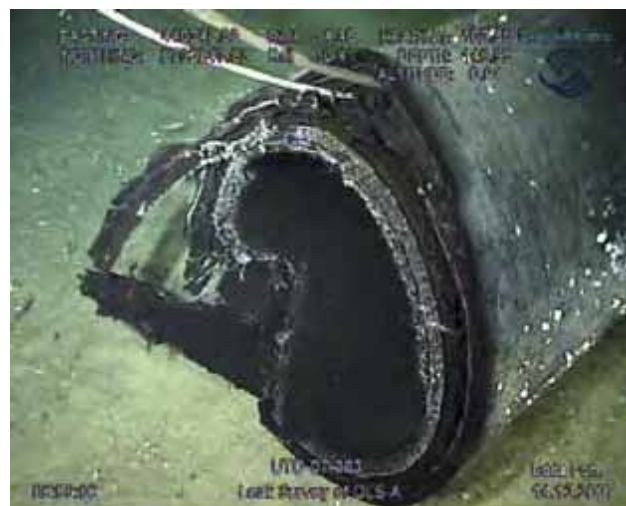
Figure 11.4 Picture of the ruptured loading hose
