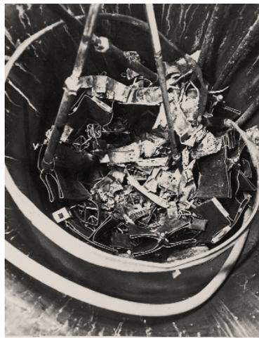
Figure 64. Damaged core resulting from steam explosion caused by a criticality accident in the military Small Low power reactor experiment SL-1 BWR. A worker inadvertently yanked out a control rod beyond the set limit during a maintenance procedure. The core became supercritical, boiled off the steam causing a steam explosion. The drying of the moderator stopped the fission reaction, even though the decay heat generation would have persisted for a while.
