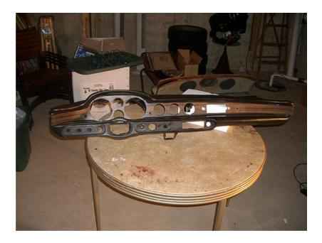
The next step is to separate the top part of the dash from the bottom. Two bolts on each end and 5 screws along the interface.
