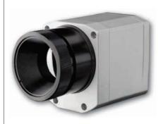
The Optris PI 640 is the smallest, most compact video graphics array infrared camera in the world. Optical resolution is 640 x 480 pixels, giving pin-sharp radiometric pictures and videos in real time. Weighing only 320 grams, it has a temperature range from -20 to 900°C, a spectral range of 7,5 to 13 μm and a frame rate of 32 Hz. Typical applications are in the surveillance, quality assurance, automotive, glass and photovoltaic industries. Visit Stand E12 to view the PI 640.
