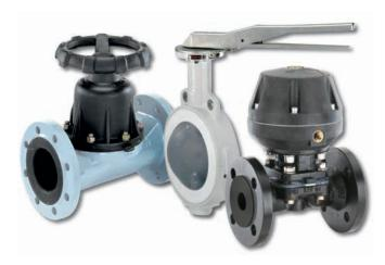
Lined diaphragm valves from Gemü can withstand both corrosive media and high temperatures. They are used in water treatment, the chemical industry, the paper industry and mining. A metal valve body with hard rubber lining can, for example, be used when processing abrasive media such as slurries from the mining industry or limestone suspensions for flue gas desulphurisation processes. View these valves at Stand D12.
