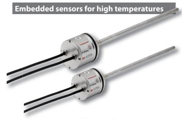
The Temposonics G-Series Model GTE embedded magnetostrictive sensors operate at temperatures as high as 85°C and feature a redundant output and IECEx Zone 2 approval for use in hazardous areas. They use an absolute measurement, which eliminates the need for regular maintenance. Magnetostrictive sensors do not require calibration and have limited moving parts. This significantly increases their reliability in even the harshest operating environments. The sensors are on view at Stand E7.
