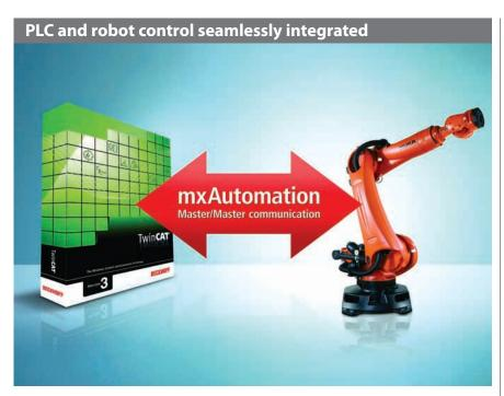
Beckhoff and Kuka are presenting a new common interface. The PLC library under TwinCAT 3.1 supports the mxAutomation interface to Kuka. Commands can be sent directly from the PLC to a Kuka robot with a KR C4 controller. It is thus possible for the first time ever to program the controller and robot simply on one system, without
