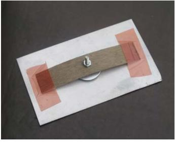
little practice determine how much adhesive required to achieve a little 'squeeze out' of adhesive around the periphery of the washer. The width of this fixture holds the stud nicely perpendicular to the surface.
