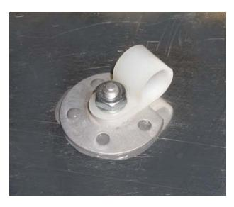
While browsing through a manufacturer's salvage outlet store some years back I discovered a part that consisted of a 10-32stud welded to a perforated flange about 1" in diameter. With the Click Bond products in mind I purchased a handful and conducted some tests with a variety of off-theshelf adhesives. The first experiment with JB Weld on thick aluminum produced a very strong bond.
