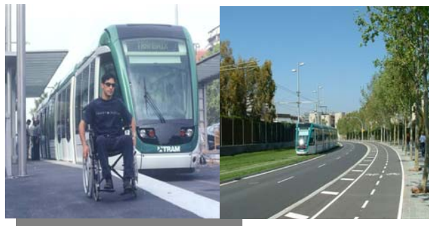
Figure 3 Aspects of the “Trambaix” tramway design: left; wheelchair access at stops, right; road space allocation showing tramway and cycle lanes.
