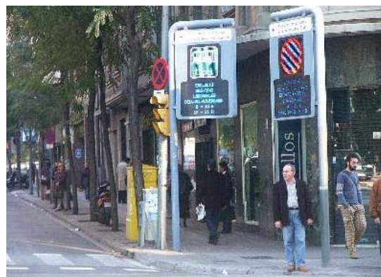
Figure 2 Left: new VMS message for bus priority Right: Trav. De Gracia lane on the left, joins with the earlier Muntaner scheme, showing a peak-hour clearway.
