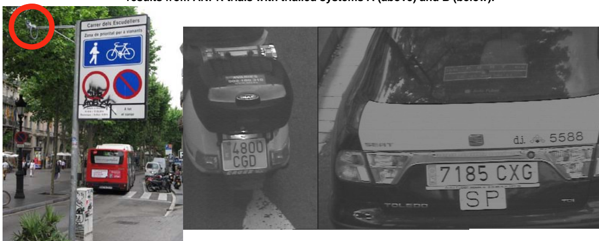
Figure 4 ANPR trials using provisional camera locations, ("entry" control point shown left) achieved sufficient read levels for car plates, but only a small fraction of PTWs. Source: SICE.
