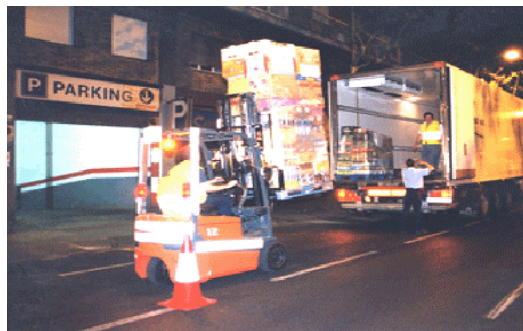
Figure 5 Quiet night-time unloading using adapted 40T truck at Mercadona's Valencia St outlet.
