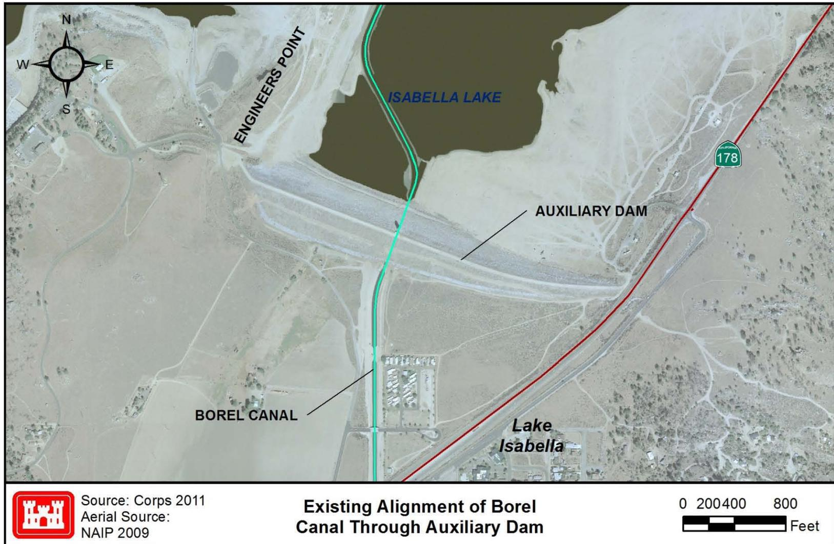
(upstream of the Auxiliary Dam) to the existing exposed Borel Canal downstream of the Auxiliary Dam (Figure 2-6-FEIS).
