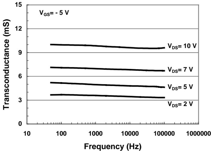
Fig. 3. Measured transconductance as a function of frequency for the  $0.25 \mu\text{m} \times 0.2$  mm device under constant gate-source bias.
