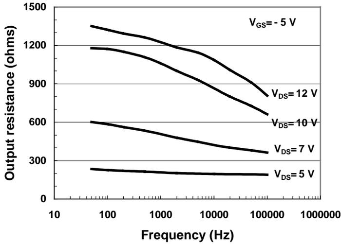
Fig. 1. Measured output resistance as a function of frequency for the  $0.25 \mu\text{m} \times 0.2$  mm device under constant gate-source bias.
