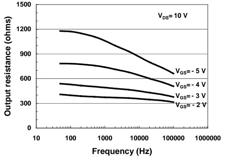
Fig. 2. Measured output resistance as a function of frequency for the  $0.25 \mu\text{m} \times 0.2$  mm device under constant drain-source bias.
