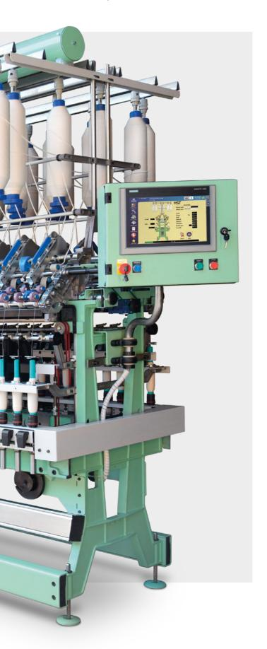
standards, letting the operator set all technological parameters, including draft and pre-draft, from touch screen. The distance from one cylinder to the other is easily settable thanks to the innovative design of the head stock.
